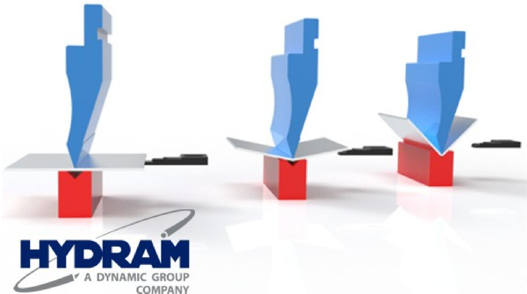
Sheet metal is bent when it is forced between two tools by the pressbrake: an upper tool (known as a punch) and a bottom tool (known as a V-die). The pressbrake controls the movement of either the punch or the die and provides the press force using hydraulic rams or electrical servo motors. The bend angle is predominantly determined by the depth of penetration of the punch within the V-die.
